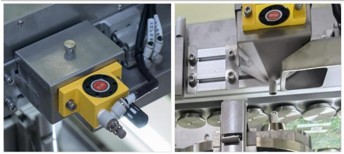
Standard with the nozzle automatic cleaning function. Strong cleaning of nozzles with cleaning powder.
