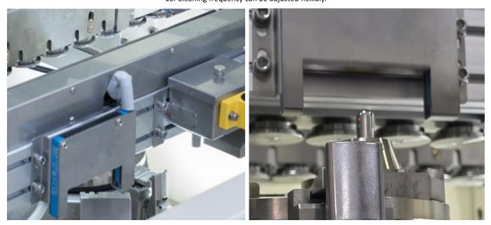
14. Laser detection system for soldering wave height.
