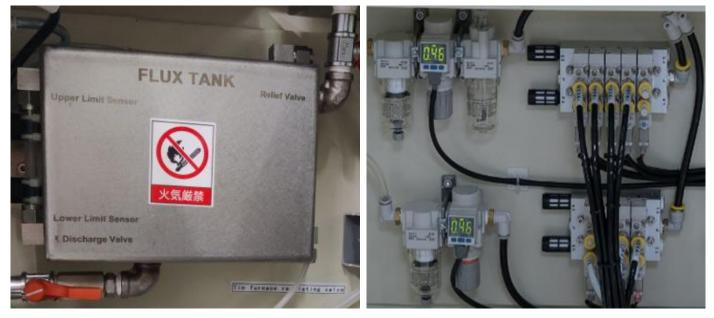
4. Flux is stocked by pressure tank, make sure pressure stable without influenced of amount of flux.
