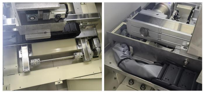
8. XYZ platform is composed of high precision lightweight sports module and high-speed servo motor.9. All servo motor are equipped with reducer to ensure stability.
