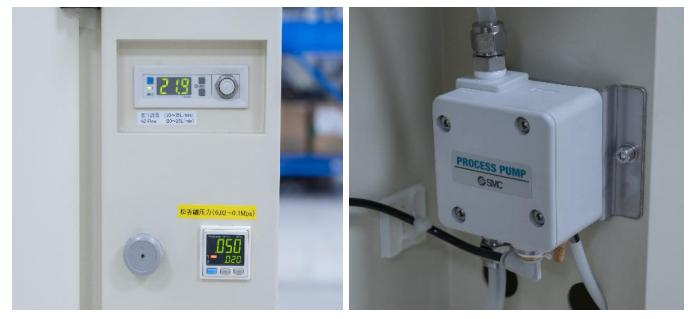
7. Flux pressure flow meter and nitrogen flow are placed on the surface of the machine for visual operation.
